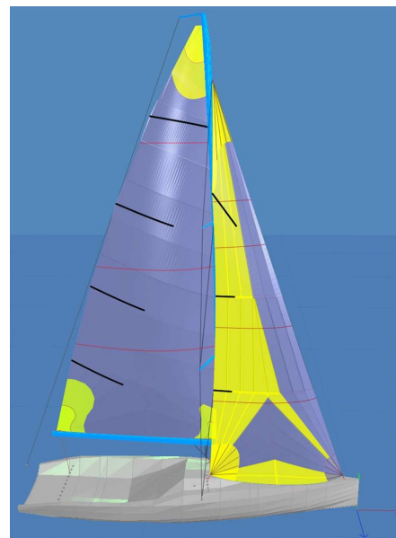
Figure 3- Representation of the sails geometry with battens and frames from CAD SailPack®
